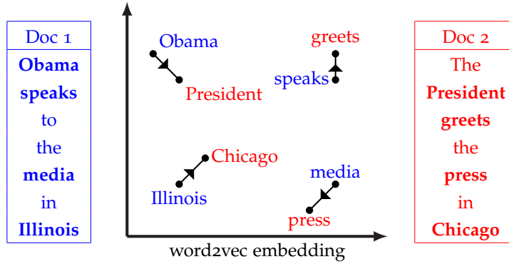
Figure 5.1: The Word Mover’s Distance by Kusner et al. (2015).
